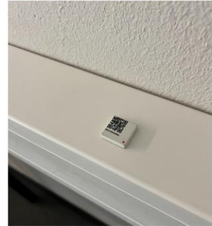
Indoor temperature sensor placed for local room measurements
