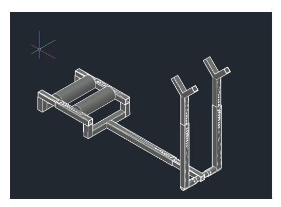
At the last stage of assembly, one of the rolls needs to be made into a lead for a current generator, with the help of which it will be possible to charge electrical devices. The drive from the roll to the generator will be made with the help of two-wheel gears and a chain.
